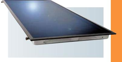
The collectors in this series consist of a deep-drawn aluminium basin, a laser-welded aluminium full surface absorber, a 50 mm thickmineral wool plate and a piece of highly translucent, hail-proof solar glass. The collectors are available in both vertical and horizontal formats.
