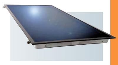
The collectors in this series consist of a deep-drawn aluminium basin, a laser-welded aluminium full surface absorber, a 50 mm thickmineral wool plate and a piece of highly translucent, hail-proof solar glass. The collectors are available in both vertical and horizontal formats.
